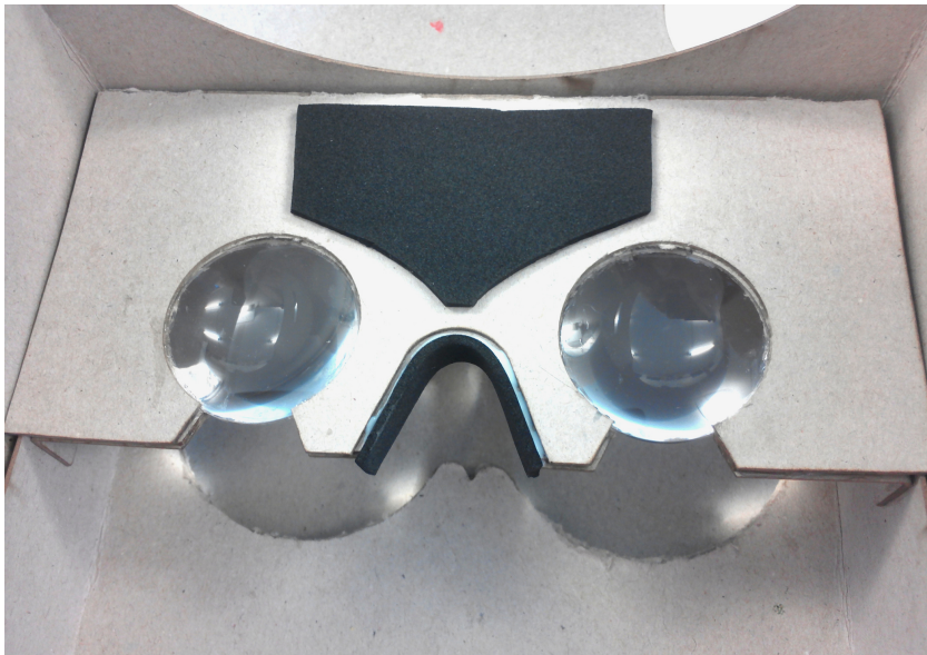
Figure 1.0.22: foam rubber attached on the cardboard
