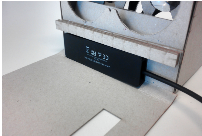
Figure 1.0.41: Position of 4-port USB-hub inside the flap
