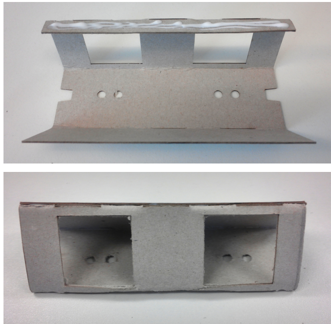
Figure 1.0.8: Glueing the connecting link to other end of the part B
